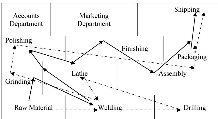
Figure 10.1.1: Typical process layout format
