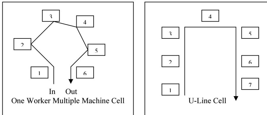
Figure 10.4.1: Example of OWMM and U-Line cell
