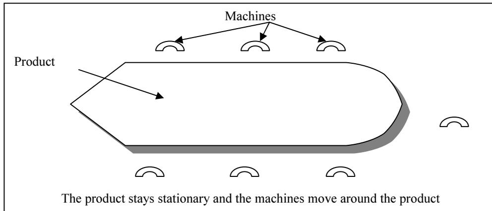
Figure 10.1.3: Typical fixed position Layout
