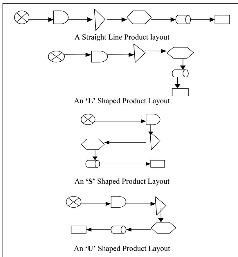
Figure 10.1.2: Typical process layout formats
